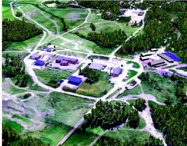
Figure 4: The Image shows a Model of an Area Generated using a Digital Elevation Model, an Orthophoto, 3D Models of Buildings and 3D Models of Single Trees.
