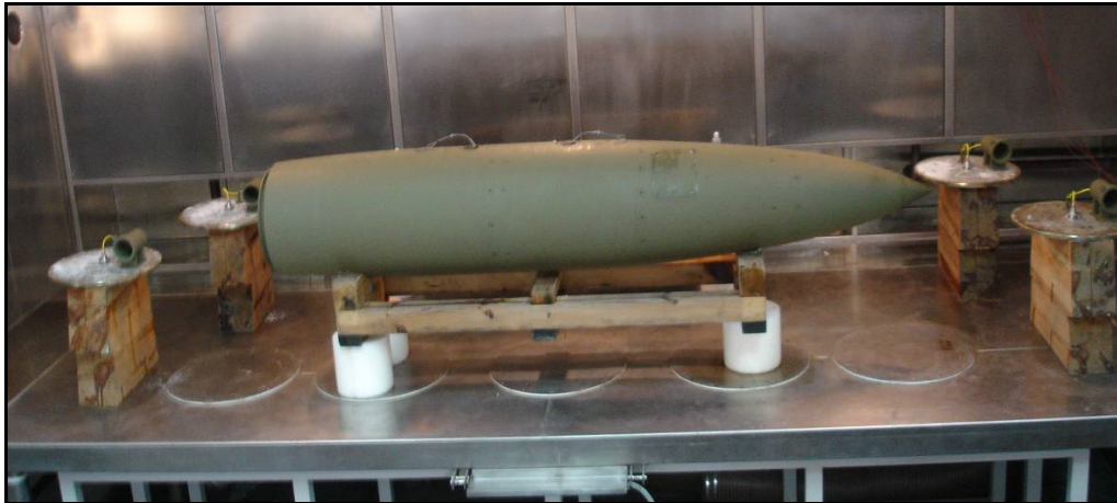
Figure 4-33: An Example of Humidity Test.
