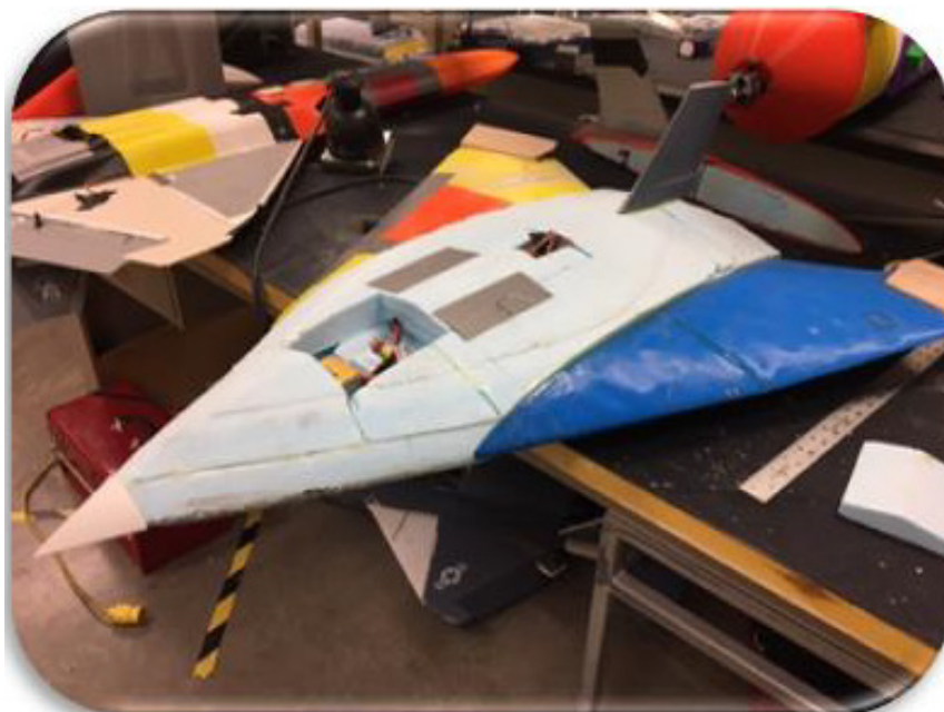
Figure 11-19: ICE 1/10th Scale Foam Test Aircraft.
