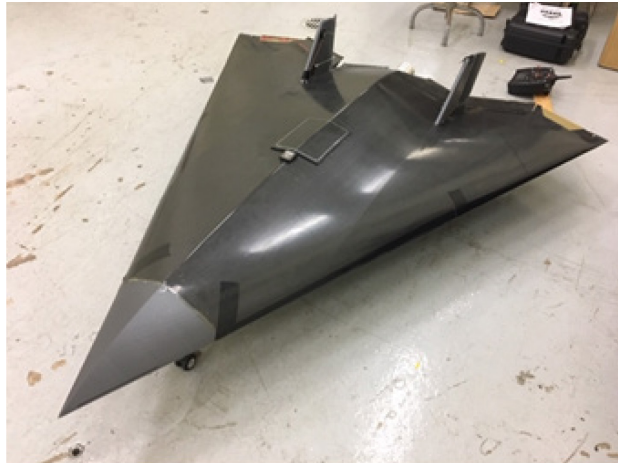
Figure 11-26: 1/7th Scale ICE Jet Powered Trainer.
