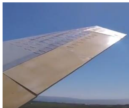
(b) Wool Tuft Measurements in-Flight at Approximately 5 Degrees Angle of Attack.
