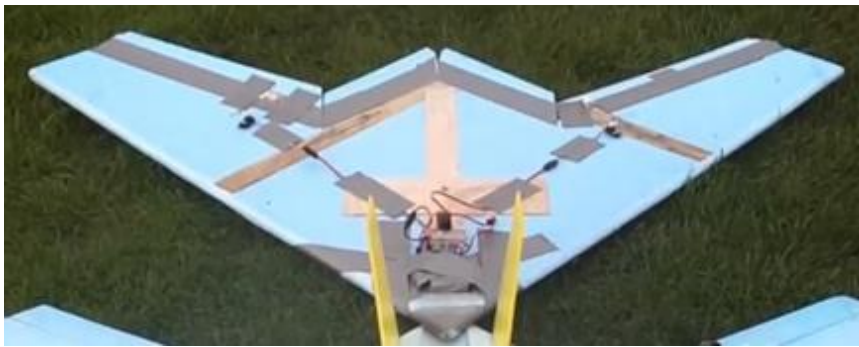
Bungee Launched 1/3 Scale, Flat Plate Model Glider.
