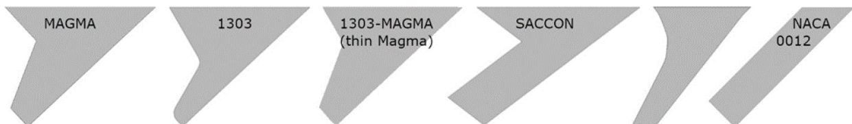
Figure 5-2: Four BWB Models (Left) and Two Swept-Back Wings (Right) Tested Using a Small Number of Sweeping Jet Actuators for the Purpose of Suppressing Spanwise Flow.
