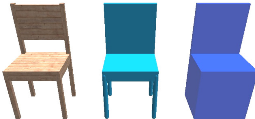
Figure E-14: Detailed Visual Model and Two Possible Versions of Simplified Collision Shapes.
