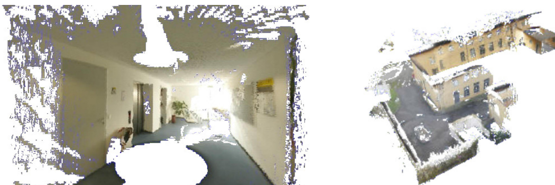
Figure E-5: 3D Reconstruction of a Real-World Scene Captured by a Mobile Robot [7].
