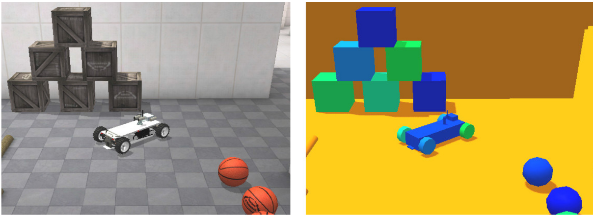
Figure E-15: Difference Between a Visual Representation of a Scene and Simplified Collision Models.
