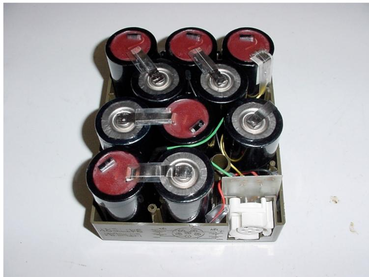
**Figure 4-2: An Example of the Lithium Primary Battery Designated BA 5590 and with the Back of the Casing Removed to Show the Internal Construction.**
