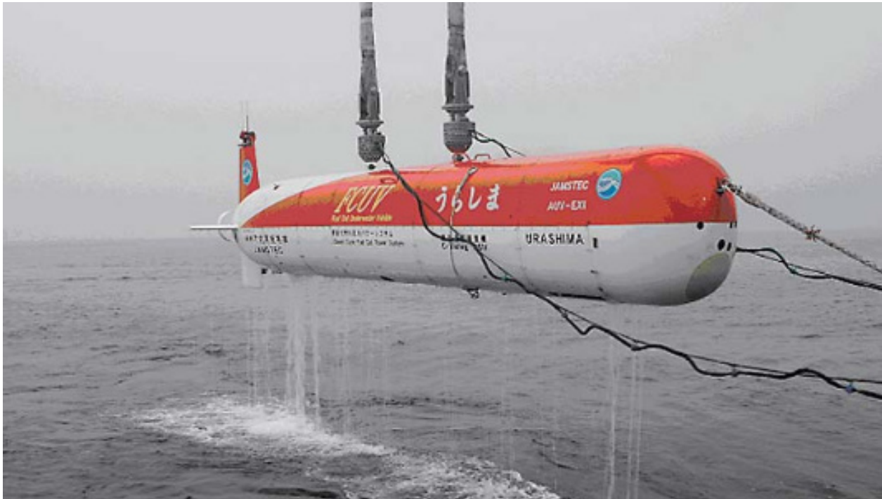
Figure 5-5: AUV Urashima Powered by Fuel Cell System.
